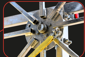
Eyelet on central spindle for ratchet strap
