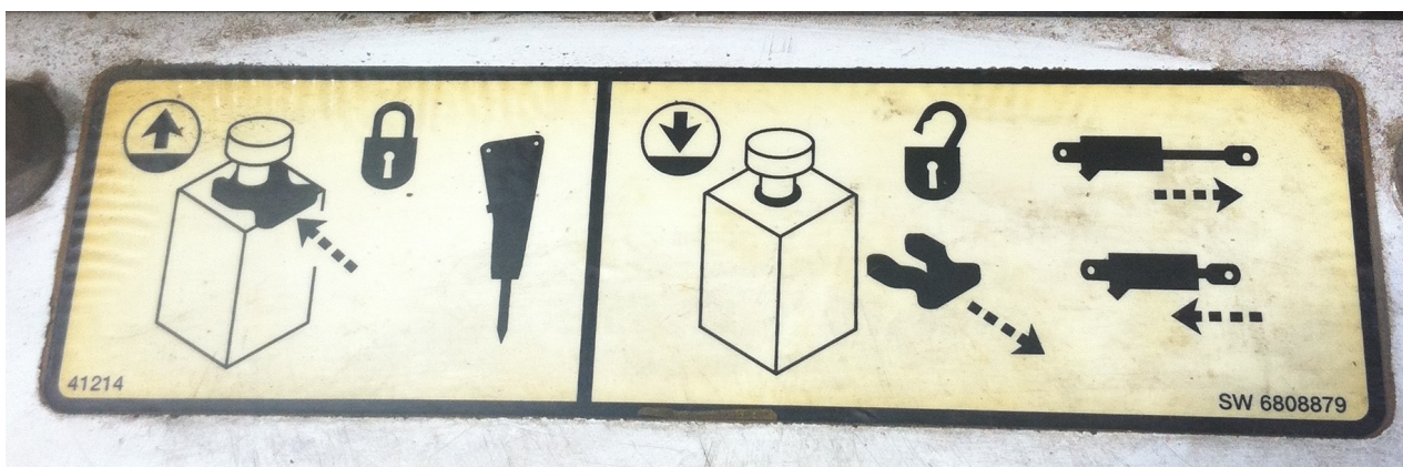
Figure 13—Typical example of a set of symbols found on a midi excavator to allow the flow of oil to be changed from single to dual flow.
