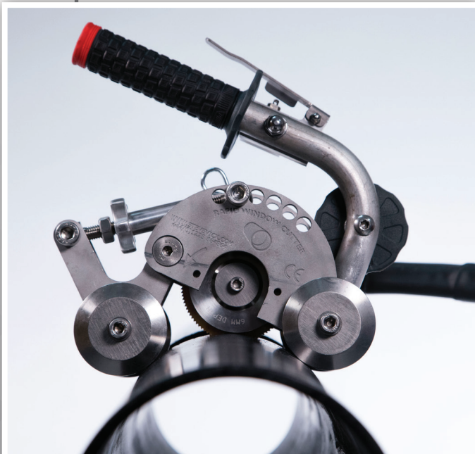
The Rapid Window Cutter for Steel mains
