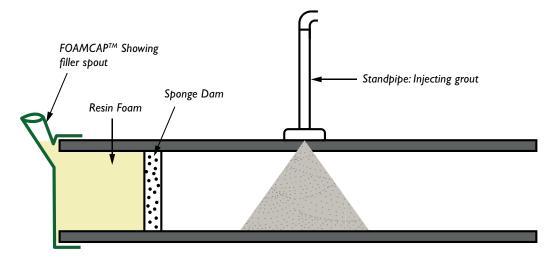
The ends of the pipe are sealed off using SVI FOAMCAPS<sup>™</sup>. The pipe is then drilled and one or more standpipes are installed through which the grout is injected.
