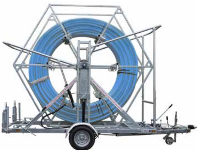
Hexi trailer with a 500m coil of 90mm PE. This model will also dispense 100m of 125mm
