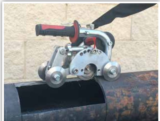
The Rapid Window Cutter for inserted ductile iron mains
