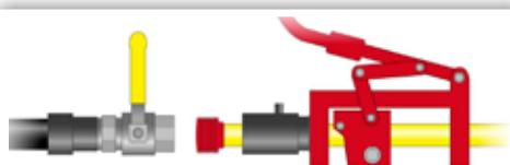
PE is inserted through valved gland assembly, replacing service under 'gas free' conditions
