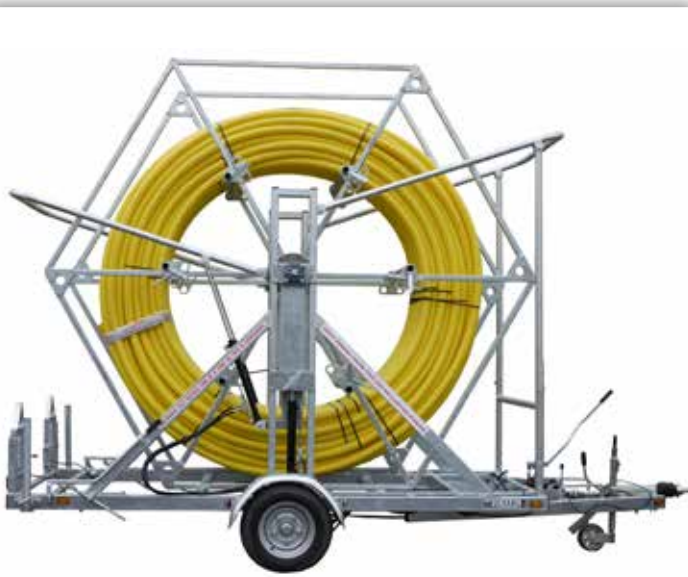
The Hexi Trailer is the first trailer of its type capable of transporting and dispensing a 500 metre coil of 90mm PE
