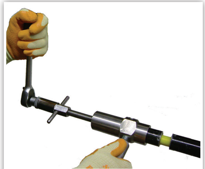
Diagram 4: The severed section of metallic pipe and cured foam sealant is pulled away
