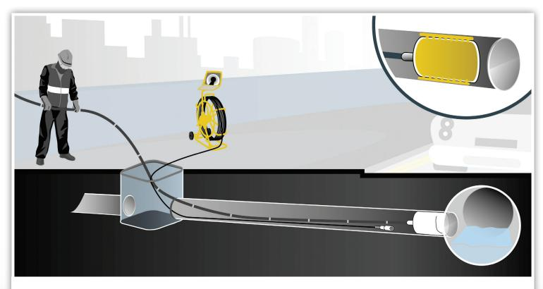
Using a CCTV and drain rods, a RATBLOCK<sup>™</sup> bag is positioned where a disused lateral drain meets the parent main. It may be installed from remote locations up to a distance of 20m or longer in certain circumstances
