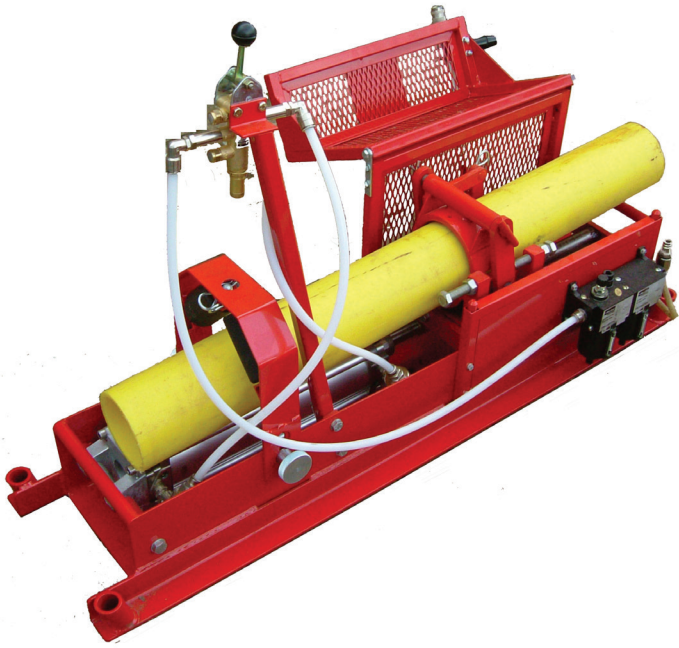
125 Pneumatic Pushing Machine for use with pipe diameters 40mm to 125mm. Max pushing speed 10 metres/minute
