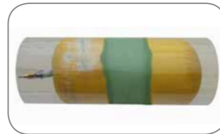
Green band appears at the points where the resin has adhered to the pipe
