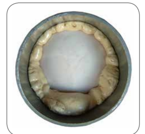
Cross section of a cured FOAMBAG™ inside a steel pipe showing how the foam seeps through the bag to adhere to the pipe wall
