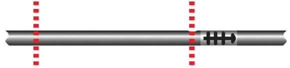
Once the Isolator Clamp is removed, the service pipe can be cut out, the first cut being made through the drilled hole near the Stopper.
