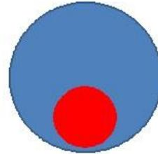
Offset Dead End Seal – used when the PE is passing through the host pipe off centre (to one side, top or bottom).
