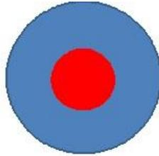
Central Dead End Seal – used when the PE is passing through the host pipe centrally.
