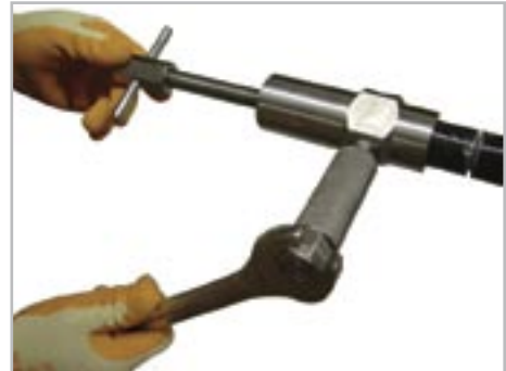
Diagram 3: The Live Service Removal Tool locked in place
