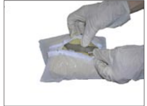
The folded sachet is then placed into the inner restraining bag with the piercing knife
