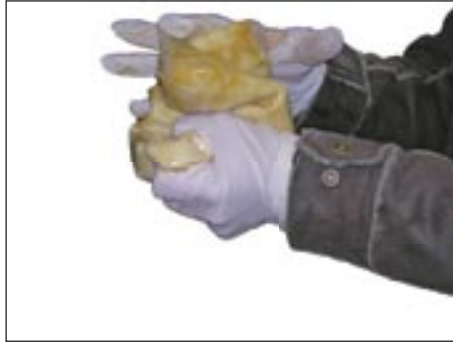
The PU resin and hardener are mixed in a sealed sachet—avoiding contact with the product
