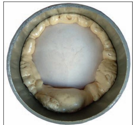
Cross section of a cured FOAMBAG™ inside a steel pipe showing how the foam seeps through the bag to adhere to the pipe wall
