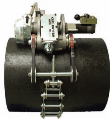
Automatic circumferential pipe cutting machine for pipe abandonment and/or diversion
