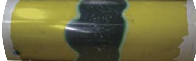
Green band appears at the points where the resin has adhered to the pipe wall
