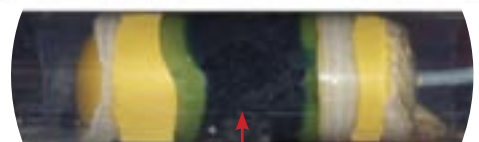
Central void filled with high performance resin
